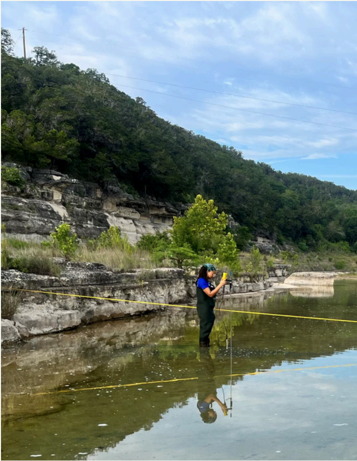
Clean Rivers Program staff collecting flow measurements
