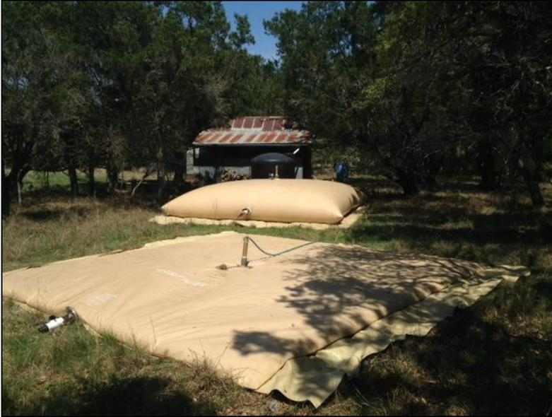
Bladder tanks for injecting water into Raccoon Cave. Each tank holds 5,000 gallons when full.
