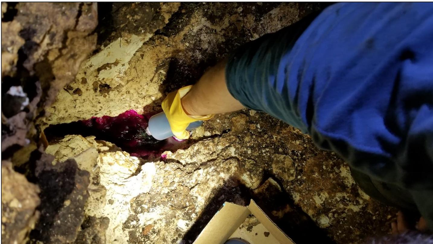
View of RWT dye as it is poured into the bottom of Raccoon Cave. Photo by Zara Environmental.
