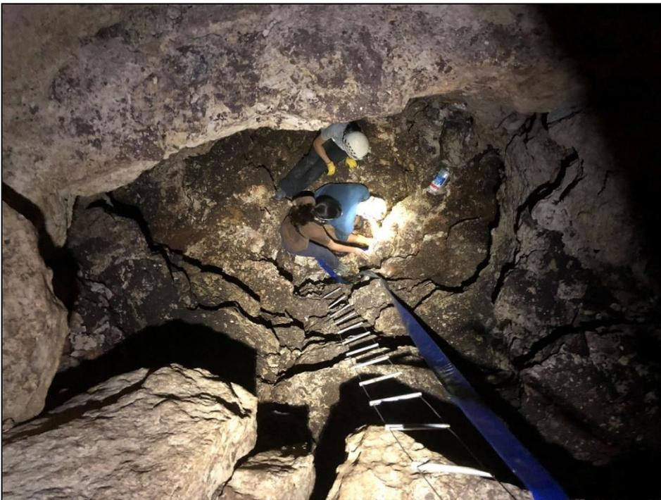
Photo looking down to base of shaft within Raccoon Cave showing the hose and injection of dye into the water flowing out of the hose.
