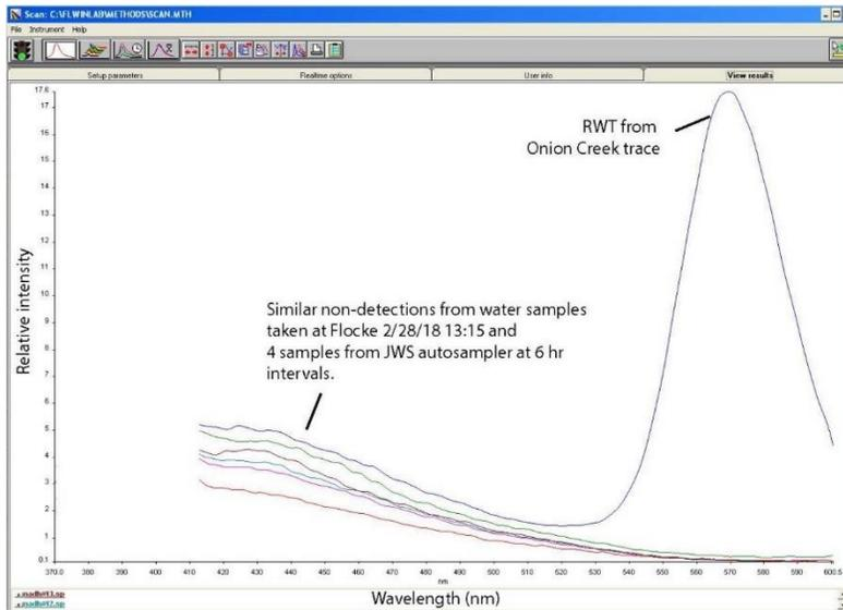
**Results from screening of water samples from JWS using the District's spectrofluorimeter. Note the flat lines are analyses from JWS and do not show a peak in the RWT range. For comparison, a positive detection of RWT is shown from another dye trace along Onion Creek.**
