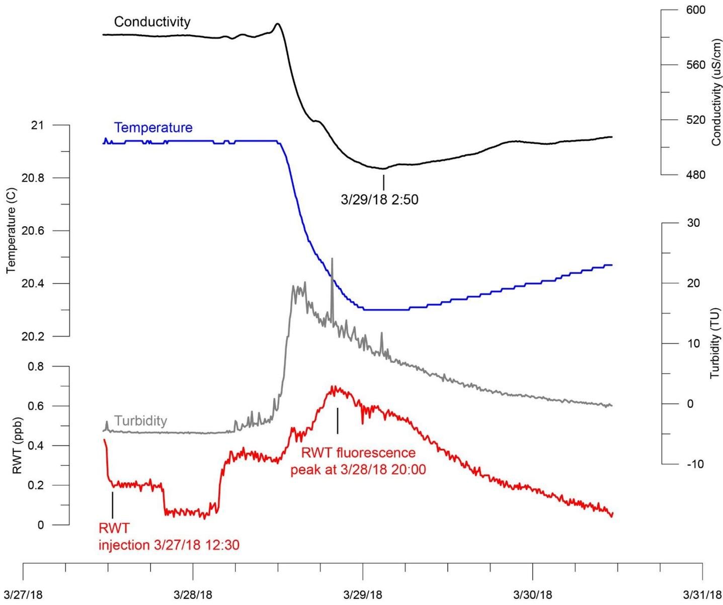
**Figure 3.** Hydrograph from the Manta2 field fluorimeter. Data frequency is 10 minutes. Field parameters responded similarly to the USGS daily data in Figure 2. Note the relative peak of RWT about 1 day after injection.
