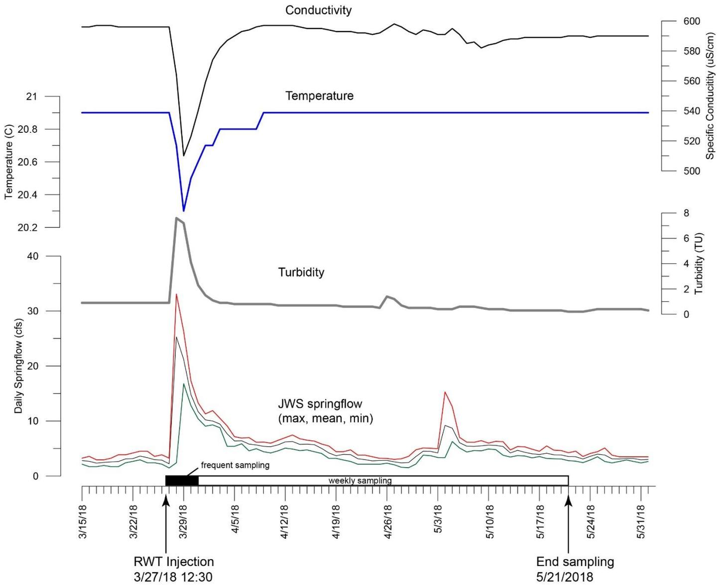
**Figure 2.** Hydrograph of USGS daily data from Jacob's Well Spring (USGS 08170990) annotated with injection and sampling notes. Rainfall occurred in the evening of 3/27/18 (after injection) and local recharge is apparent on the hydrograph resulting in increased springflow and turbidity, and decreased temperature and conductivity.
