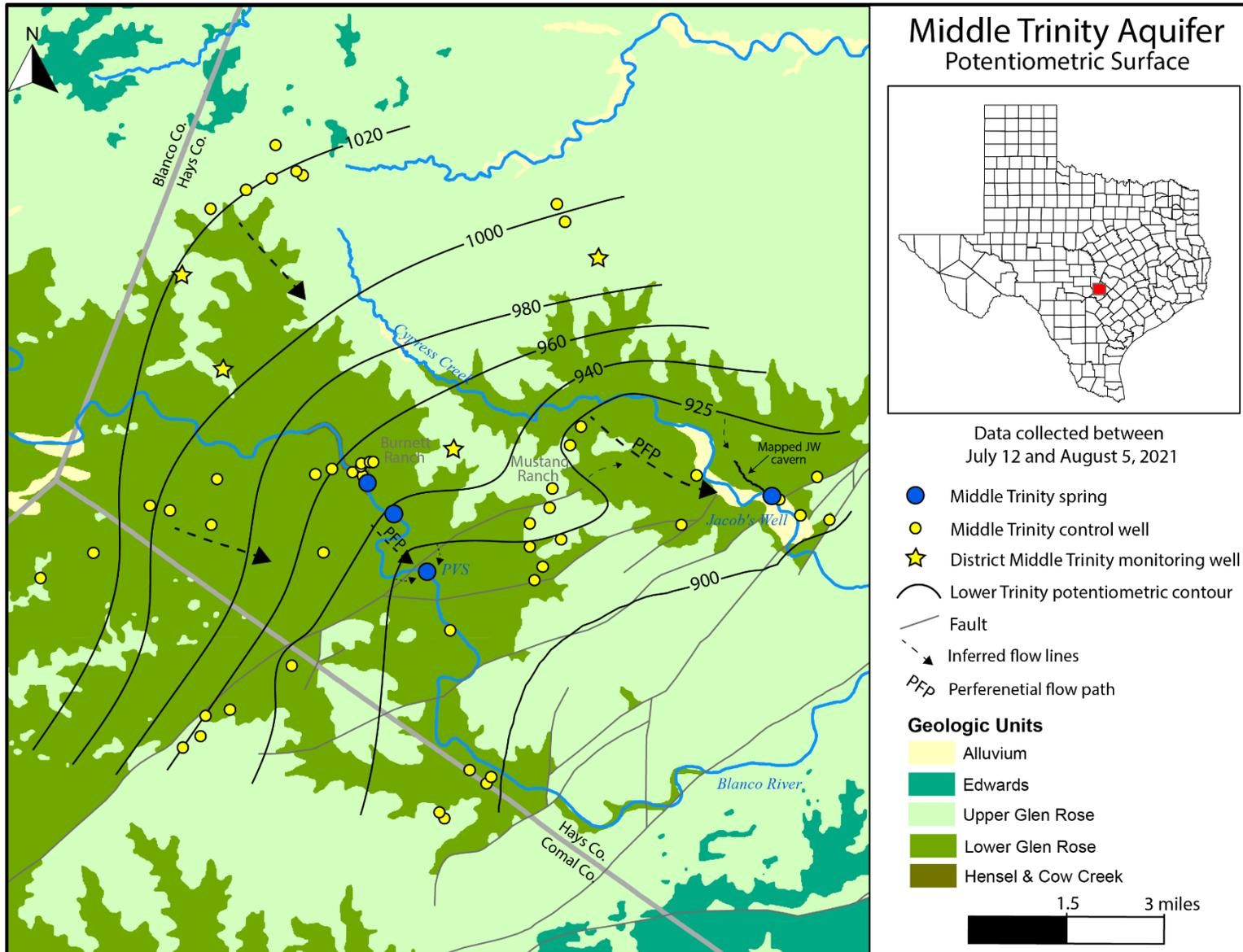
Figure 3. Middle Trinity Aquifer potentiometric surface map. Faults and geologic units from BEG (2014).
