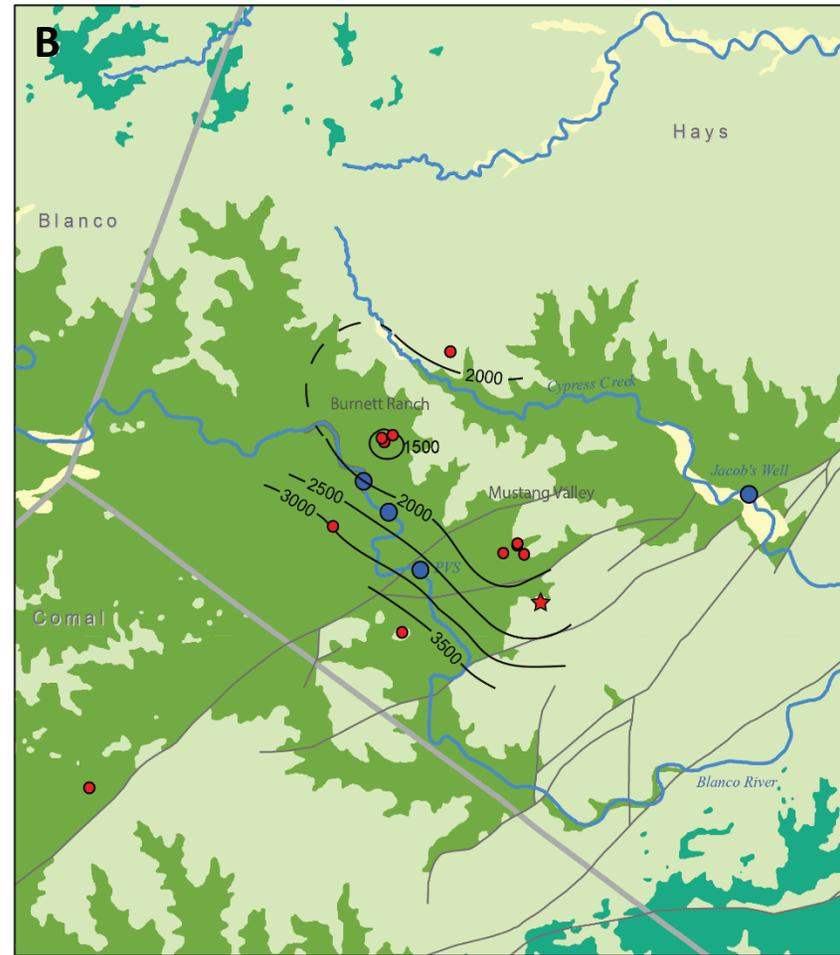
**Figure 6.** Middle Trinity (A) and Lower Trinity (B) TDS contour maps. Control wells are labels with measured TDS value. All data collected between July 12 and August 5, 2021. All values were calculated from field conductivity measurements using a correction factor of 0.64. Faults and geologic units from BEG (2014).
