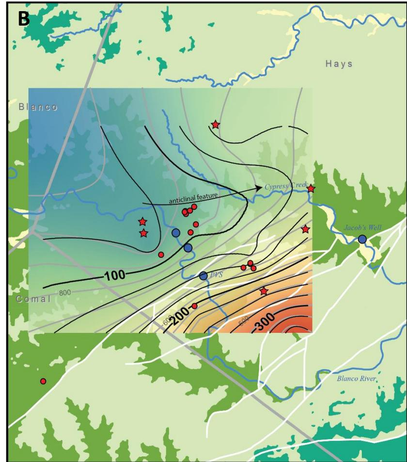
**Figure 4.** Feet of hydraulic head above the top of the Cow Creek Formation (A) and Sligo Formation (B). Shaded gradient (blue indicating higher, red indicating lower) with grey contours represents top of Cow Creek (A) and top of Sligo (B) and white lines representing faults. Arrow indicates anticlinal structure. All water elevation data collected between July 12 and August 5, 2021. Faults and geologic units from BEG (2014).
