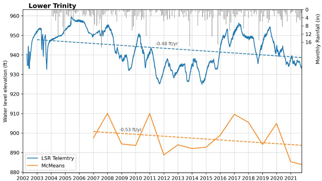
**Figure 9.** Hydrograph of District monitor wells LSR Telemetry and McMeans with monthly rainfall on the secondary x-axis. The LSR Telemetry is within the Burnett Ranch region and the McMeans well is just south of the Mustang Ranch region.
