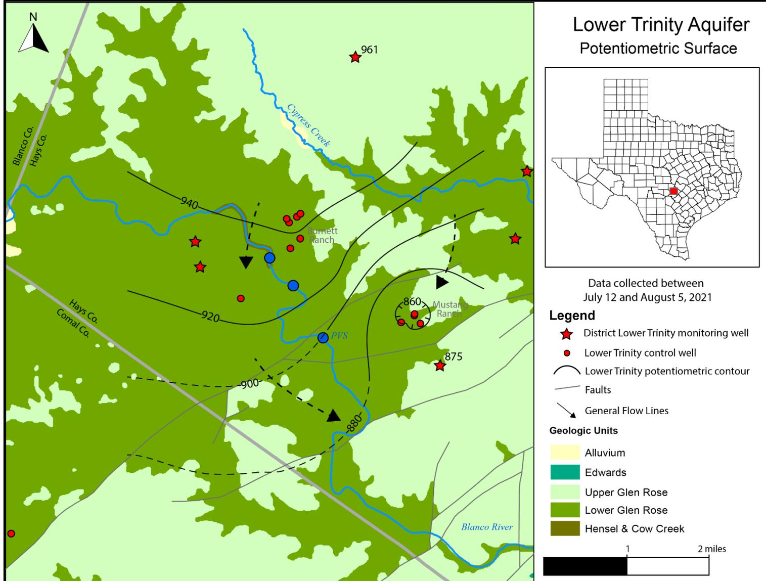
**Figure 5.** Lower Trinity Aquifer potentiometric surface map. Furthest updip and downdip control points labeled. Faults and geologic units from BEG (2014).
